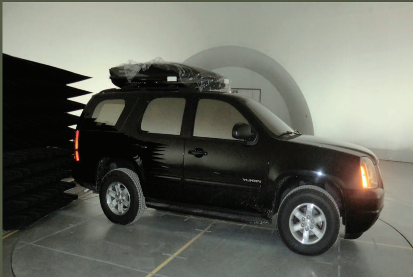
Measurement radome - interior view Vehicle placed for RF shielding measurements on rotating platform
