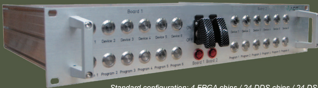
Standard configuration: 4 FPGA chips / 24 DDS chips / 24 DSP chips
